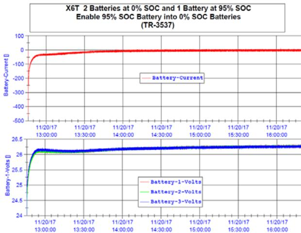
**Figure 5:** Parallel connection testing of fully charged Xcelion® 6T-Energy with two fully discharged batteries. Battery current displayed in Amps.
