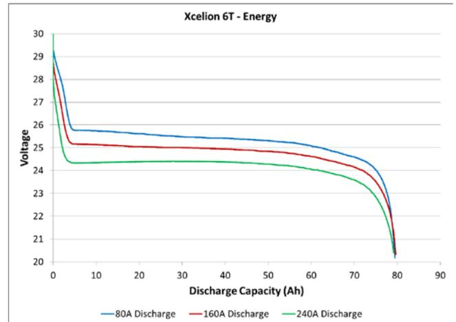
**Figure 1:** Rate Capability of Xcelion<sup>®</sup> 6T-Energy at Room Temperature
