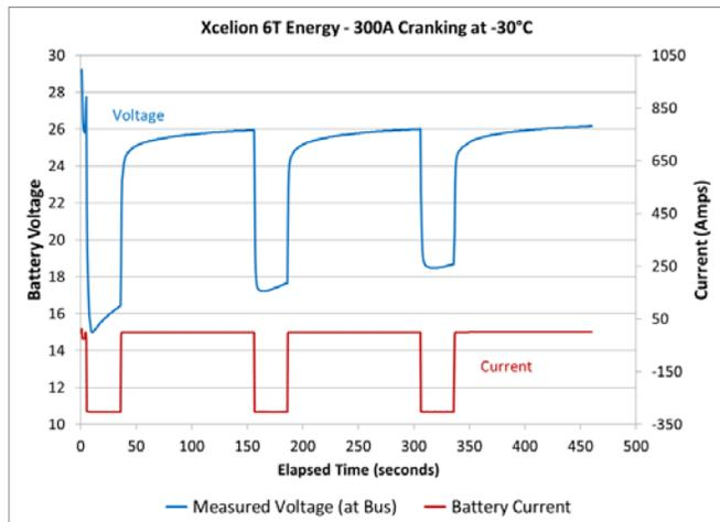
**Figure 3:** Xcelion<sup>®</sup> 6T-Energy performance under 300A/s30sec load at -30°C without preheating
