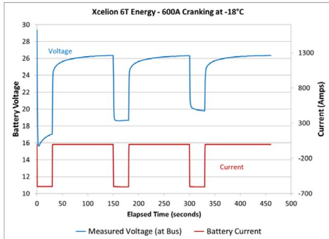
**Figure 2:** Xcelion® 6T-Energy performance under 600A/30sec load at -18°C without preheating
