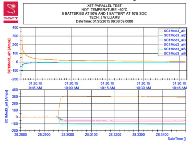
**Figure 6:** Parallel connection testing of five charged Xcelion 6T® batteries with one discharge battery
