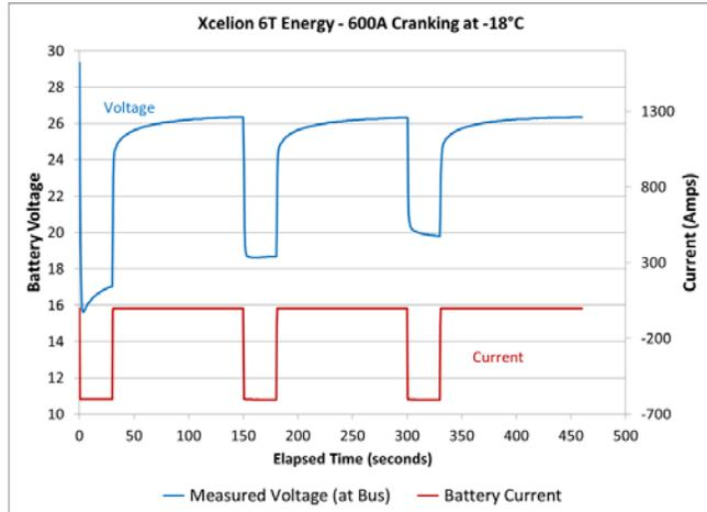
**Figure 2:** Xcelion<sup>®</sup> 6T-Energy performance under 600A/30sec load at -18°C without preheating
