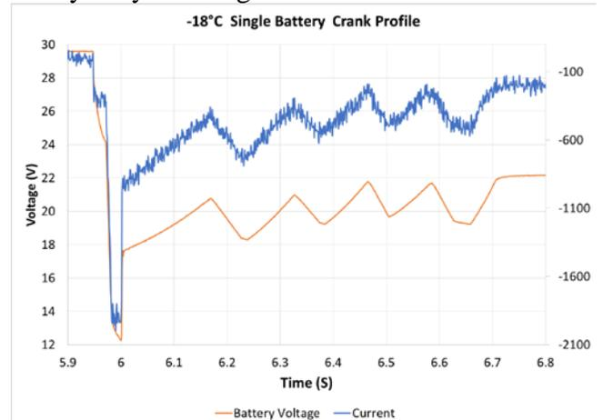
**Figure 4:** Vehicle cranking supported by a single Xcelion® 6T-Energy battery at -18°C without preheating
